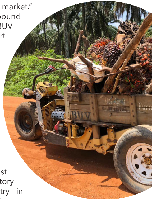
Basic Utility Vehicles carry heavy agricultural loads over bumpy roads.
